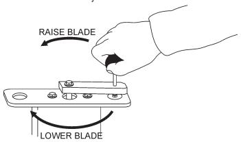
Figure 37. Blade Height Adjustment
